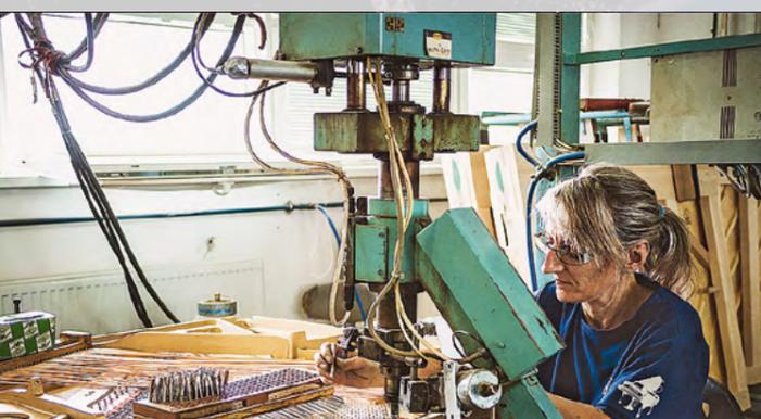
The stringing is one of the most exacting operations. The drawing of the strings onto the piano frame is partly carried out using a machine that ensures the correct height of the tuning pins and the required number of turns for the strings.
