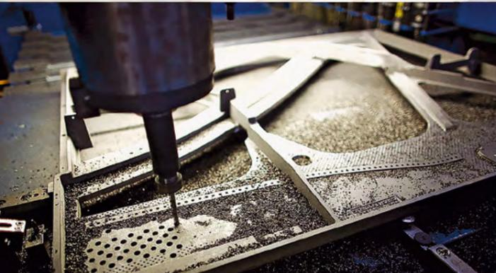
In order to achieve maximum precision, over 500 functional openings in the iron frame are drilled using a computer-controlled machine. Once it is ready, the iron frame is then polished and varnished in our factory achieving its final shape.
