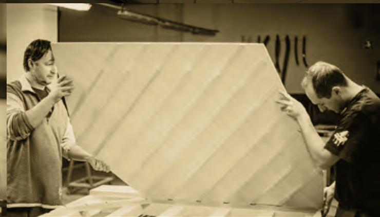
Gluing the soundboard onto the backframe.
