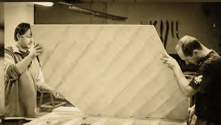
Gluing the soundboard onto the backframe.
