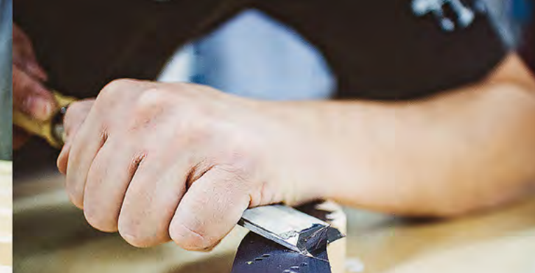
Shaping of the bridges, known as "notching", is carried out with maximum precision by our skilful workers with the use of chisels. Notches with piano bridge pins, together with agraffes, determine a very important parameter, the string scale. For this reason, great care is taken in shaping the bridges.
