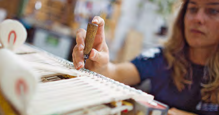
The regulation of the piano action is carried out in the PETROF factory by the most experienced employees, who have many years of practice behind them. This guarantees that the action is perfectly balanced across the entire keyboard, enabling precise interaction between the player and the instrument.
