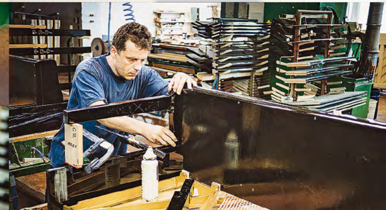
The bonding of the piano cabinet to the acoustic element, which consists of the piano framework with the iron frame and the strings. The quality of the bonding significantly affects the final appearance of the whole instrument.
