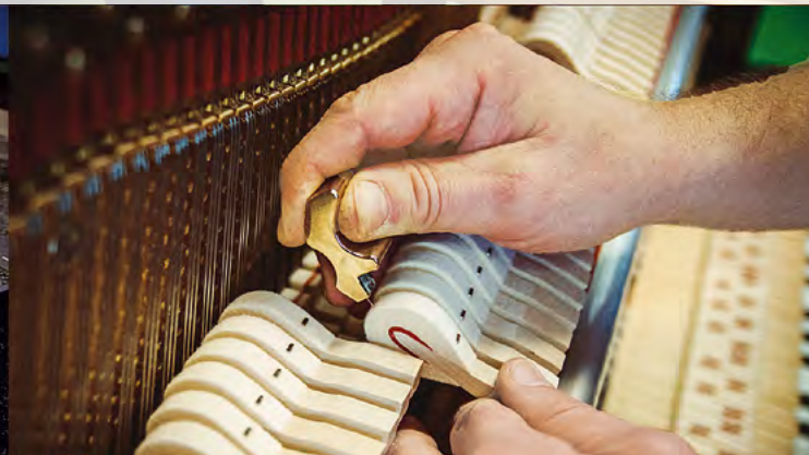
Voicing is carried out so as to ensure that every key obtains the required mechanical properties. This creates an open, colourful tone, romantic in character, which is a typical feature of PETROF instruments.
