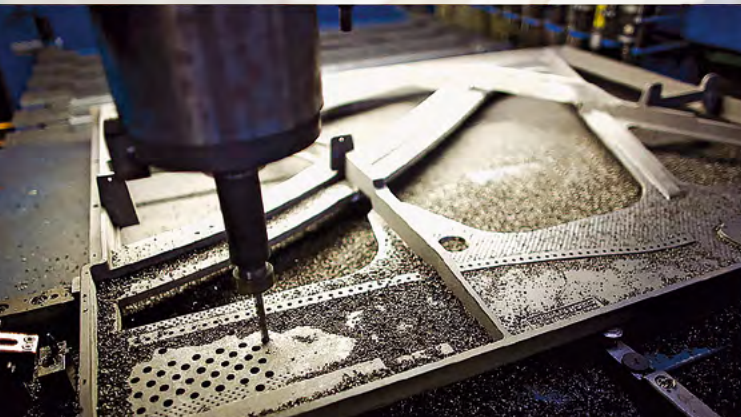
In order to achieve maximum precision, over 500 functional openings in the iron frame are drilled using a computer-controlled machine. Once it is ready, the iron frame is then polished and varnished in our factory achieving its final shape.
