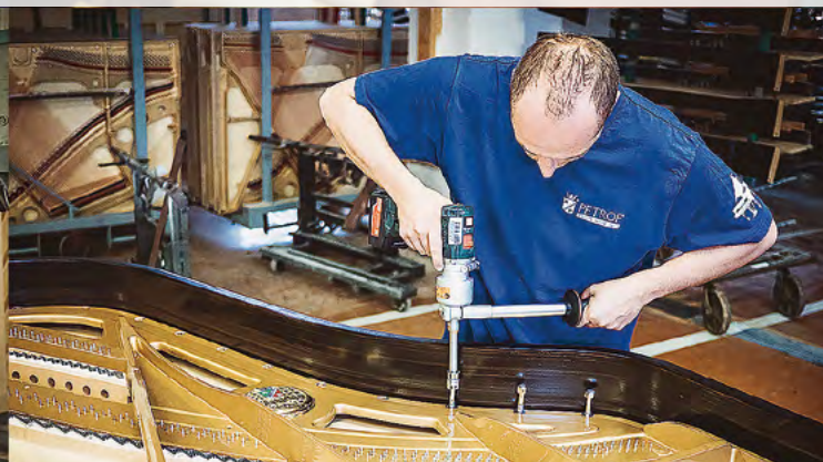
The iron frame and the wooden framework are combined by being screwed together. The iron frame must be attached to the framework very firmly, as the tension in the strings, which this construction has to bear, can in a grand piano reach over 20 tonnes.
