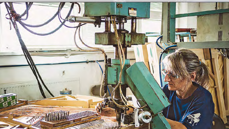
The stringing is one of the most exacting operations. The drawing of the strings onto the piano frame is partly carried out using a machine that ensures the correct height of the tuning pins and the required number of turns for the strings.
